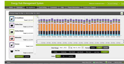
Figure 1. Appliance Level Data Screenshot of the electricity consumption for a hub as a function of the individual appliances, where each bar represents one day, and each colour represents a different appliance.
